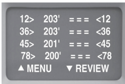
Figure 6-26. A correct wire map for a straight through cable.
